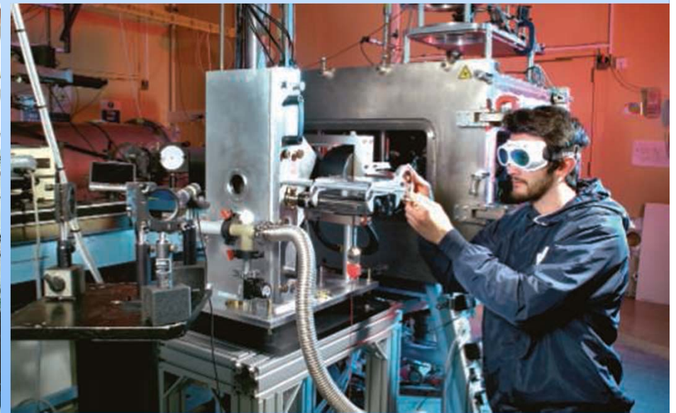
LARGE AND SMALL: (Left) Conventional accelerator at CERN. (Center) Part of the linear accelerator beamline. (Right) Benchtop laser particle accelerator for multi- MeV experiments.
