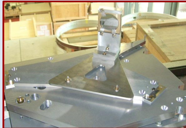
Adjusting the base plate by means of a laser mirror on tripod
