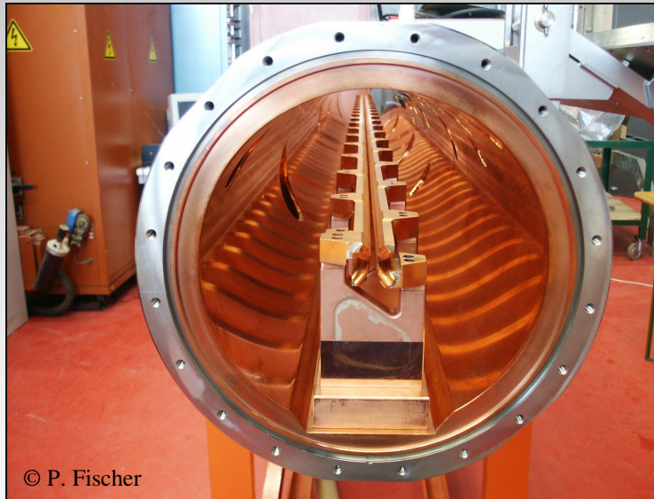
view inside of the RFQ
