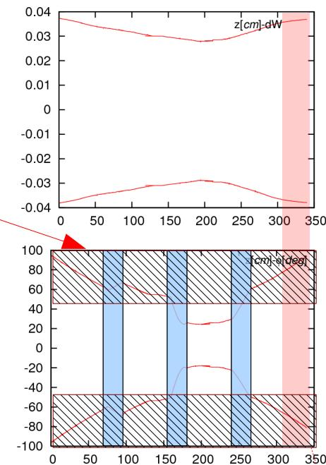
Particles in this region are not taken into account for space charge calculation in the case of static lattice size.
